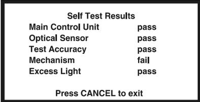
After each test, a **pass** or **fail** is displayed on the screen. If any results **fail**, the unit will not operate. Refer to Section 10 Troubleshooting.
