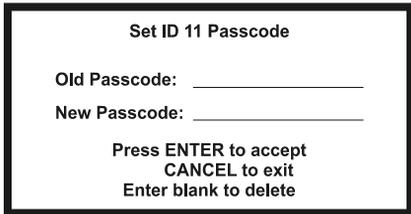
Scan or enter a new **Passcode**. Press **ENTER** to save the settings and exit. Press **CANCEL** to cancel the settings and exit. Enter a blank **Passcode** to disable the ID.
