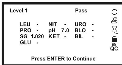
If any parameter is out of range, it will be highlighted and marked with a “\*”.
