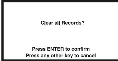
Press **ENTER** to delete all records. A prompt will appear. Once records are deleted they cannot be recovered. The **Test Number** will reset to 000001, 100001 or 200001 depending on the Test Mode. Press any other key to cancel. The screen will return to the **Database Menu**.
