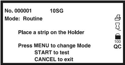
Press **START** again to begin strip testing. The strip is tested the same as other single test modes. The results screen will show the sample ID in the **ID** field.
