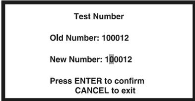
Enter the new **Test Number**. Press **ENTER** to confirm. Press **CANCEL** to delete any changes and keep the existing number.
