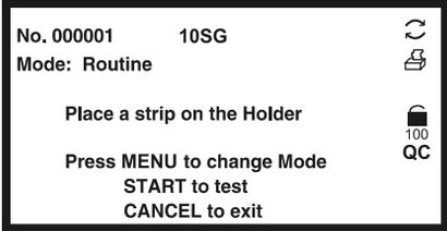
**Note:** Timing is set up to process a new strip every 30 seconds.
