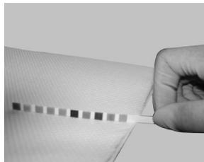
Place the strip with the reagent area facing up, onto the Strip Holder Channel. Make sure the strip end touches the Strip Holder Backstop as shown below.
